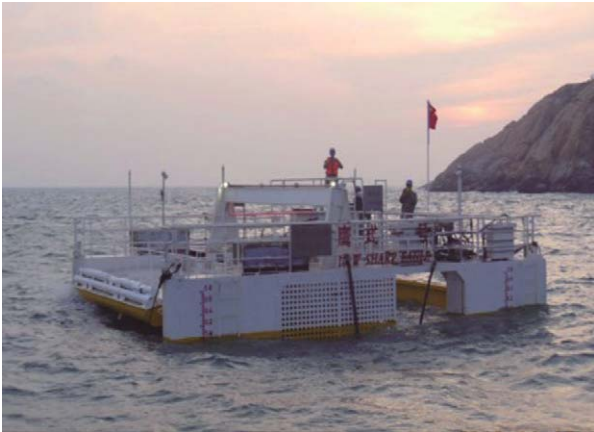
Fig. 5. The 10 kW Eagle WEC developed by GIEC.
