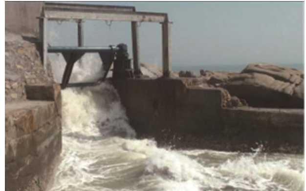
Fig. 3. The 30 kW pendulum WEC developed by NOTC.
