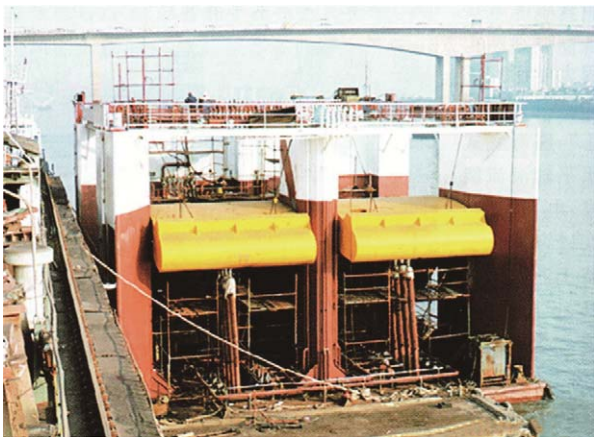
Fig. 6. The 150 kW Eagle WEC developed by GIEC.
