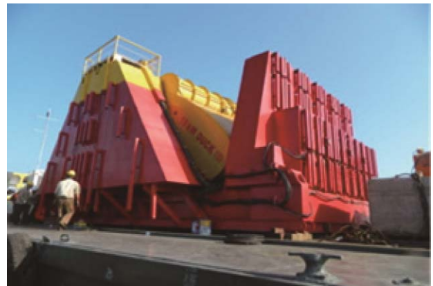
Fig. 4. The 100 kW nodding duck WEC developed by GIEC.
