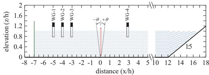
**Fig. 3. Model setups and normalized coordinate system from Chen et al. (2014)**
