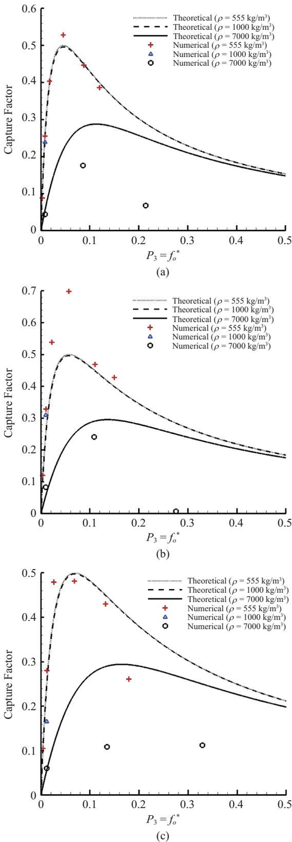
Fig. 5. Comparisons of capture factor between theoretical and SPH results for cases of three densities of the flapper body ( $\rho = 555, 1000, 7000 \text{ kg/m}^3$ ) at wave periods of (a)  $T = 1.11 \text{ sec}$ , (b)  $T = 1.33 \text{ sec}$ , and (c)  $T = 1.57 \text{ sec}$ .
