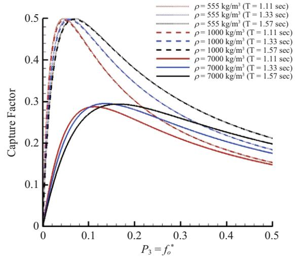
**Fig. 4. Variations of theoretical capture factor with the PTO-damping impedance ( $P_3$ ) or the dimensionless damping coefficient of PTO for cases of three periods of incoming wave ( $T = 1.11, 1.33, 1.57$  sec) and three densities of the flapper body ( $\rho = 555, 1000, 7000$  kg/m<sup>3</sup>).**
