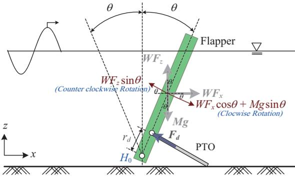
Fig. 2. Definition sketch of the bottom-hinged flapper.
