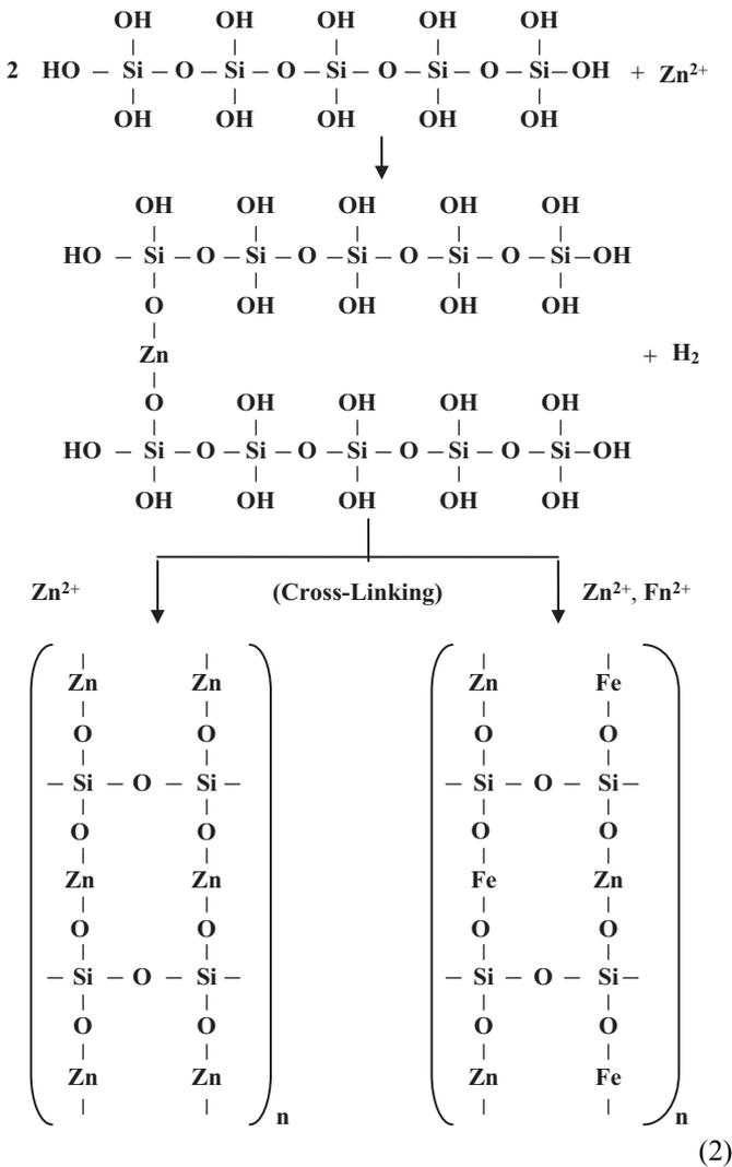
Consequently, a solid film with zinc-silicate-zinc and zinc-silicate-iron compounds is generated (Fig. 1).
