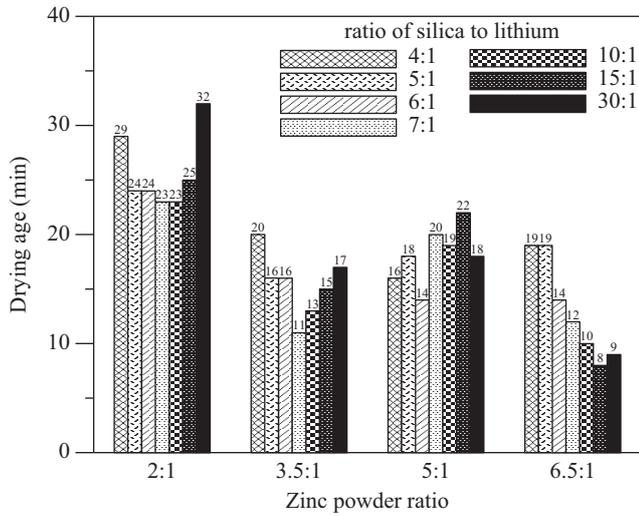
Fig. 2. Drying times for the various mixtures.
