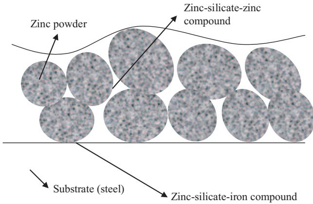
Fig. 1. Crosslinking effects generated zinc-silicate-zinc compounds and zinc-silicate-iron compounds.
