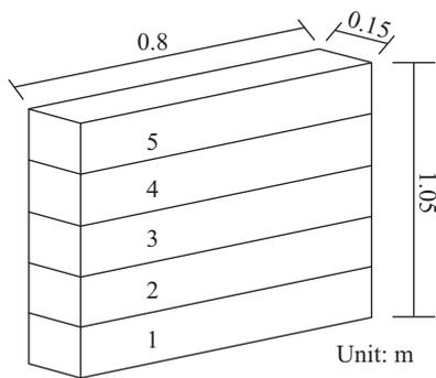
**Fig. 2. Bottom-hinged plate and its dimensions (unit: m).**
