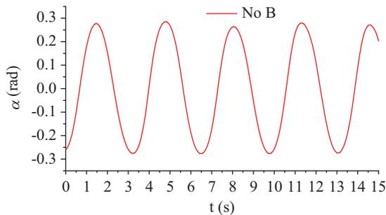
Fig. D. Time histories of the flap rotation angle  $\alpha$  with  $T_{pto} = 75$  Nm at  $T = 3.13$  s,  $A_i = 0.067$  m.
