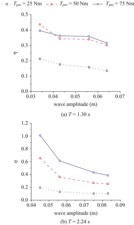
Fig. 5. Variations of capture width ratio  $\eta$  vs wave amplitude for different damping torque.
