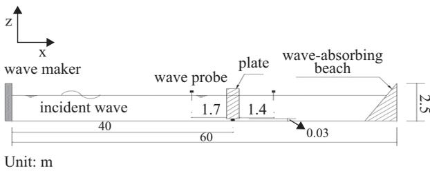
**Fig. 1. Schematic of the experiment (unit: m).**
