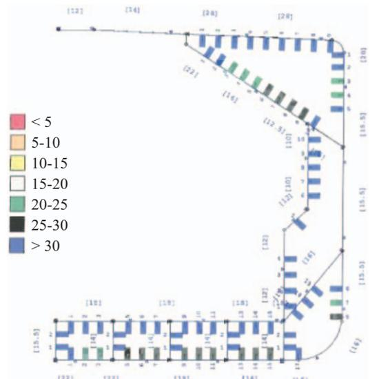
Fig. 7. Calculated fatigue life (years) expectancies of longitudinal stiffener end connections at a transverse bulkhead.
