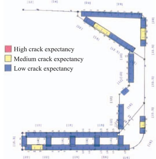
Fig. 9. Inspection guidance for longitudinal stiffener end connections at bulkheads in the midship area.
