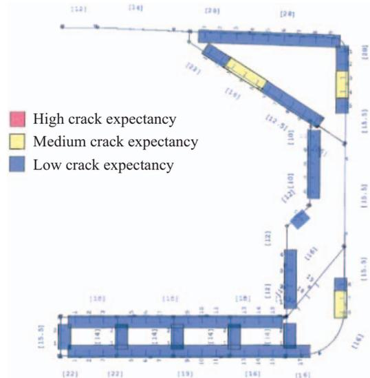
Fig. 8. Inspection guidance for longitudinal stiffener end connections at ordinary frames in the midship area.
