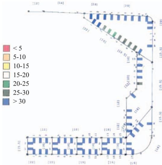
Fig. 6. Calculated fatigue life (years) expectancies of longitudinal stiffener end connections at a typical frame in the midship area.
