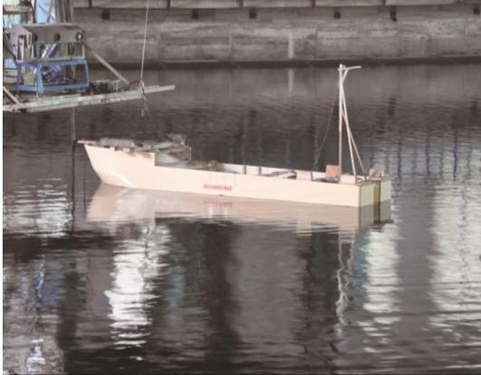
Fig. 3. Roll decay test of HYSY201 vessel model.
