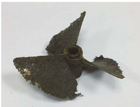
Fig. 16. The worn propeller after 16 months of operation.
