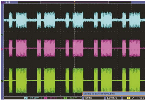
Fig. 13. Transmitter output signals (blue: codec output, pink: amplifier card output, green: main board output).
