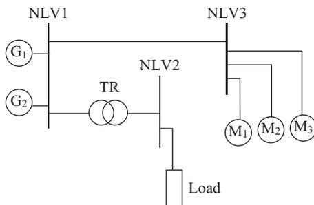
**Fig. 5. The equivalent electric single wire diagram of research operation (operation condition 4).**
