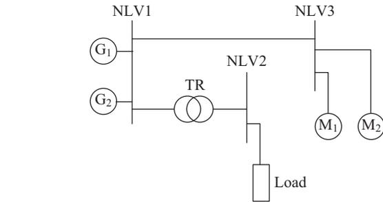
**Fig. 2. The equivalent electric single wire diagram of entering and leaving port (operation condition 1).**
