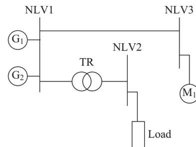
**Fig. 3. The equivalent electric single wire diagram of entering and leaving port (operation condition 2).**
