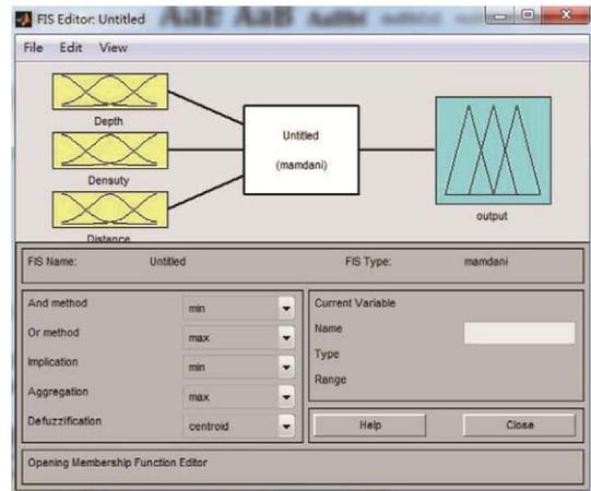
**Fig. 8. Membership function input & output system.**
