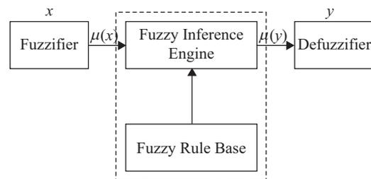
Fig. 2. Basic framework of a fuzzy control system.
