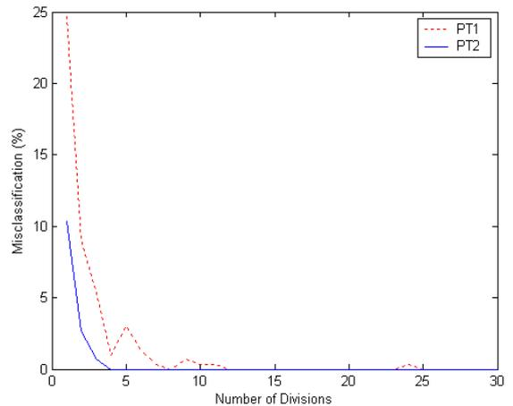
**Fig. 3.** Misclassification versus the number of partitions on the frequency axis for the 15 fault cases with the STFT and the unit STD method being used.
