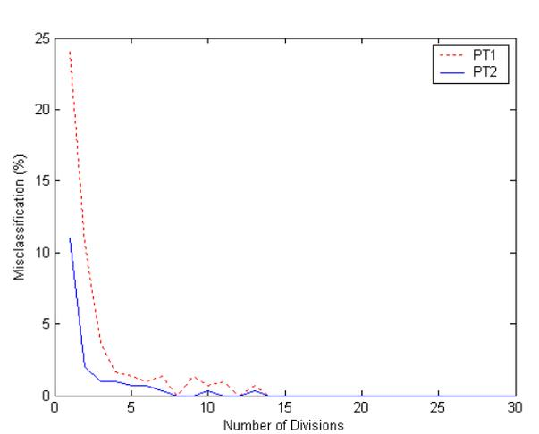
**Fig. 9.** Misclassification versus the number of partitions on the frequency axis for the 15 fault cases with the RSPWVD and the unit STD method being used.
