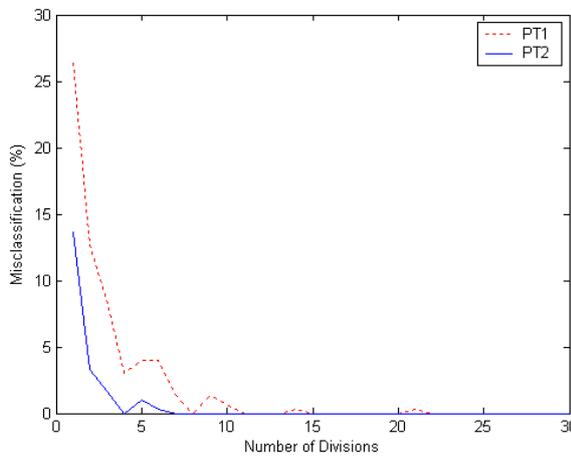
**Fig. 5.** Misclassification versus the number of partitions on the frequency axis for the 15 fault cases with the SPWVD and the min/max method being used.
