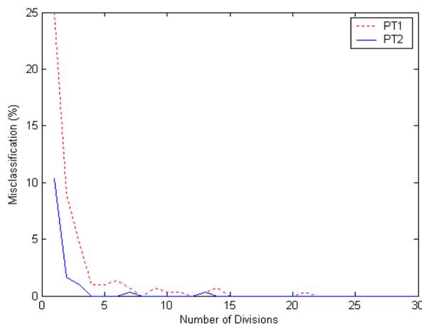
**Fig. 6.** Misclassification versus the number of partitions on the frequency axis for the 15 fault cases with the SPWVD and the unit STD method being used.
