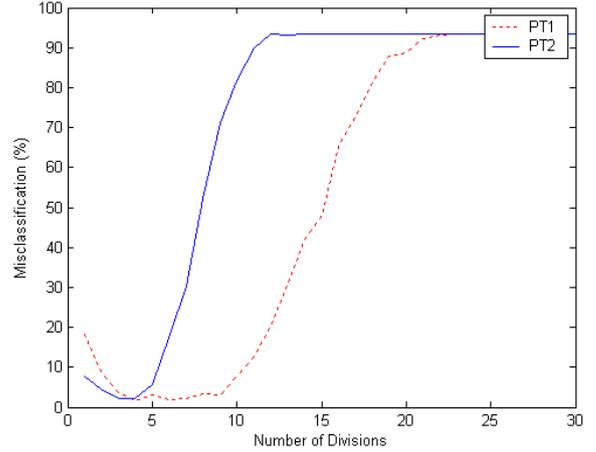
**Fig. 1.** Misclassification versus the number of partitions on the frequency axis for the 15 fault cases with the STFT and the mean variation method being used. PT1 (No. of Partitions on the Time Axis: 1), PT2 (No. of Partitions on the Time Axis: 2)
