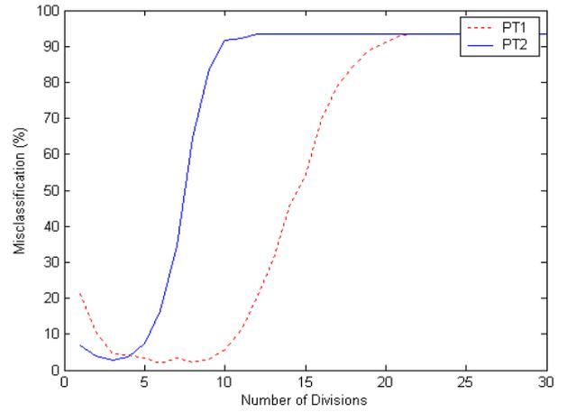
**Fig. 7.** Misclassification versus the number of partitions on the frequency axis for the 15 fault cases with the RSPWVD and the mean variation method being used.
