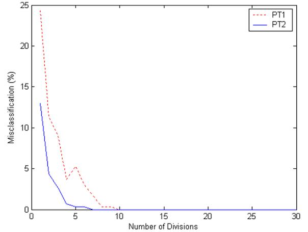
**Fig. 2.** Misclassification versus the number of partitions on the frequency axis for the 15 fault cases with the STFT and the min/max method being used.
