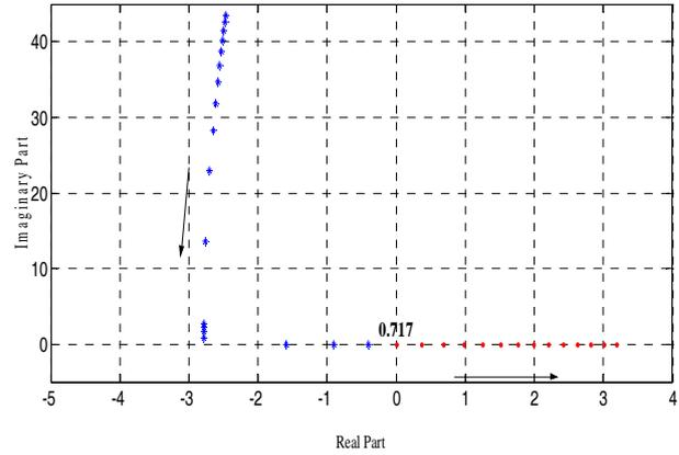
Fig. 3. The second mode root loci in the vicinity of the divergence instability as the rotation angle, ' $\theta$ ', of the left eigenvector changes while the modal control weight  $E_{s22}^{-1}$  remains fixed.
