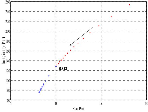
Fig. 4. The second mode root loci in the vicinity of the flutter instability as the rotation angle,  $\theta$ , of the left eigenvector changes while the modal control weight  $E_{s22}^{-1}$  remains fixed.
