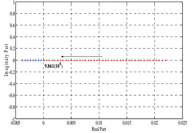
Fig. 7. The second mode root loci in the vicinity of the upper bound divergence instability as the modal control weight  $E_{s22}^{-1}$  changes while the left eigenvector remains fixed.
