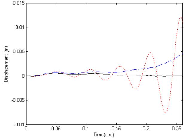
Fig. 2. Tip responses for different rotation angles of the left eigenvector with  $E_{s22}^{-1}$  being fixed.
