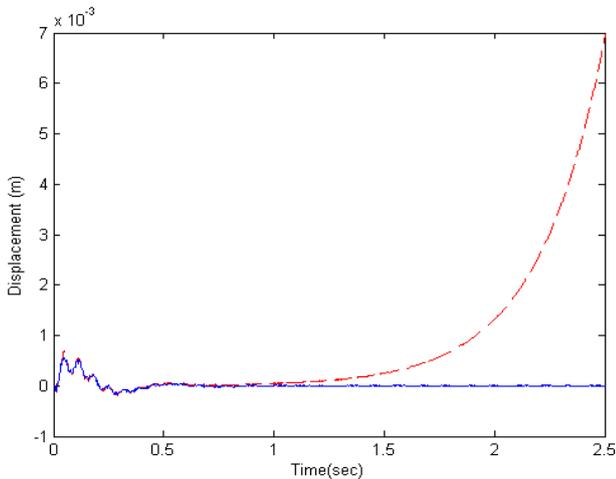
Fig. 5. The controlled and uncontrolled tip responses with a fixed baseline left eigenvector, illustrating divergence instability.
