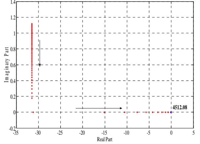
Fig. 6. The second mode root loci in the vicinity of the lower bound divergence instability as the modal control weight  $E_{s22}^{-1}$  changes while the left eigenvector remains fixed.
