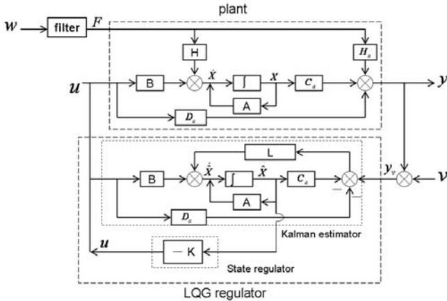
Fig.2 Block diagram of LQG control system
