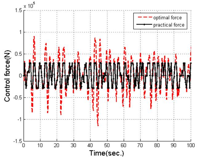
**Fig.5 MR damper force compared with optimal force**
