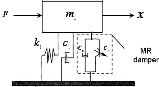
Fig.1. Schematic diagram of a SDOF platform coupled with a MR damper
