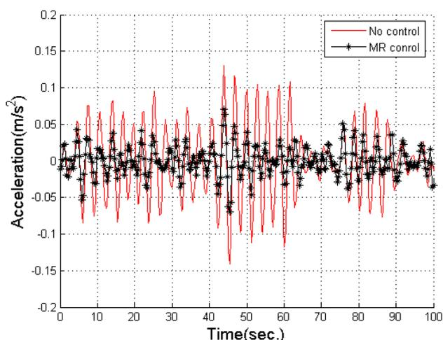
Fig.7 Acceleration of the platform
