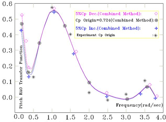
Figure (12): effect of  $C_p$  variation on vessel pitch motion in different frequencies
