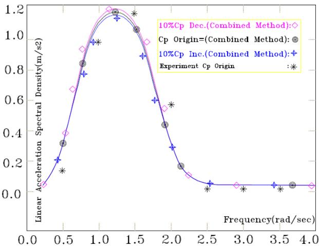
Figure (13): effect of  $C_p$  variation on vessel pitch motion in different frequencies
