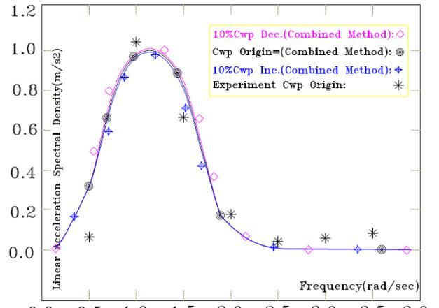
Figure (19): effect of  $C_{wp}$  variation on vertical acceleration in different frequencies
