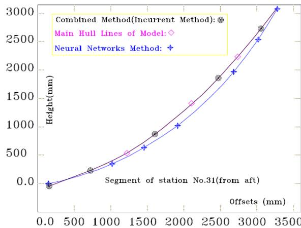
Figure (4): difference of modeled vessel transverse section by combined method (neural networks method and polynomial fitting), main hull lines form and neural networks method
