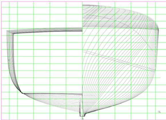
Figure (6): vessel model body lines
