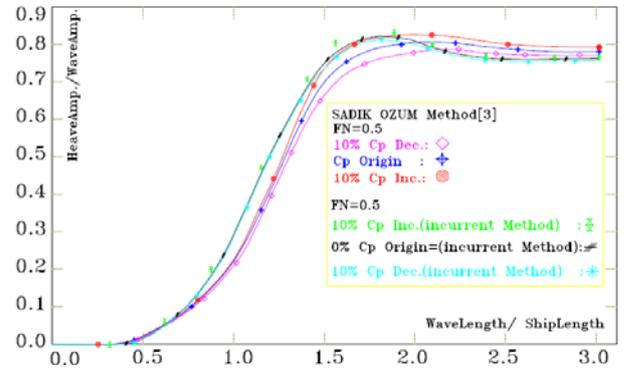
Figure (15): comparison of  $C_p$  variation effects on the vessel heave motion for 8% increase, 8% decrease and main model with  $C_p$  maintained from Ozum *et al.* [12] method.
