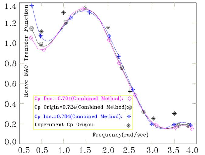
Figure (10): effect of  $C_p$  variation on vessel heave motion in different frequencies
