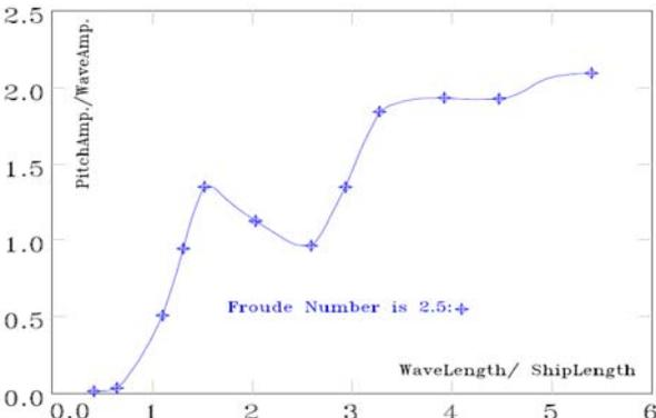
Figure (9): vessel pitch amplitude in wave amplitude of 2 cm
