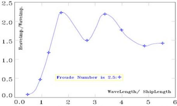
Figure (8): vessel heave amplitude in wave amplitude of 2 cm
