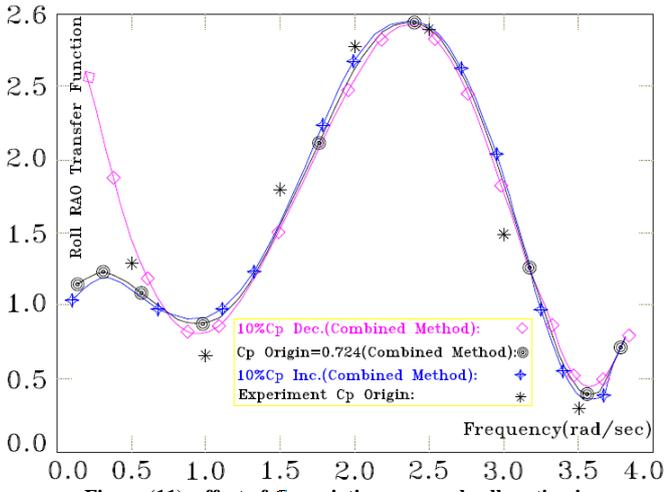
Figure (11): effect of  $C_p$  variation on vessel roll motion in different frequencies
