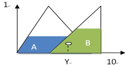
Fig 5 Gravity method schematically
