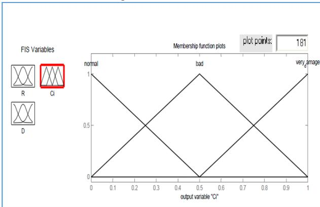
Fig 4 Inference output membership function Parameters
