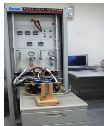
Fig. 6. Performance test equipment of PEMFC
